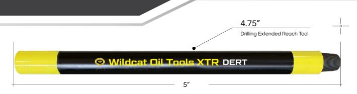
7.0 Tool **Tool Size** 4.75" Overall Length 54" Temperature Range 150-320F Weight 75 lbs **Operational Flow Range** 1 - 5 BPM Pressure Range (Static) 10,000 psi Operational Frequency 8 Hz @ 168 gpm **Max Tensile** 85,000 lbs Pressure Pulse 500 - 2,300 psi
